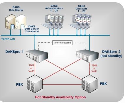
Parallel Operation with Redundancy Servers – Each operational DAKSpro server has an assigned hot standby. This topology offers the highest availability through load sharing and balancing, and through the use of hot standby servers.
